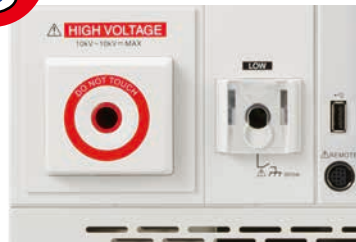
▲ Front output terminal
